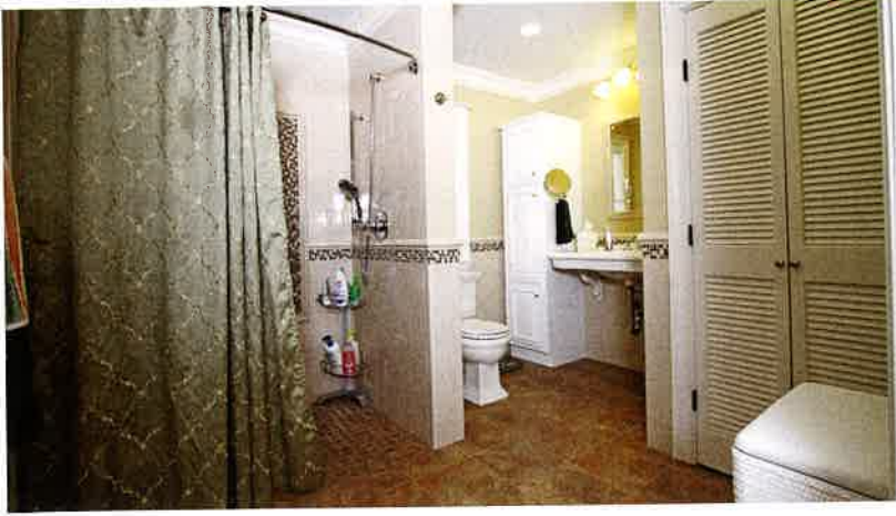
A comfortable bathroom for anyone was especially designed for a wheel chair bound daughter with roll under sink and roll in shower
